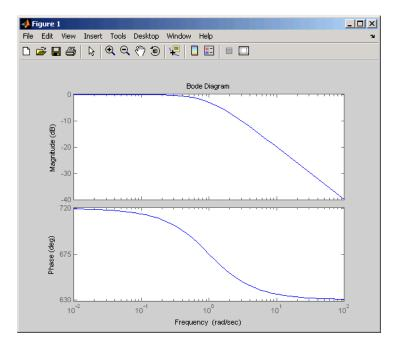
The first bode plot has a phase of -45 degrees at a frequency of 1 rad/s. Setting the phase matching options so that at 1 rad/s the phase is near 750 degrees yields the second Bode plot. Note that, however, the phase can only be -45 + N\*360, where N is an integer, and so the plot is set to the nearest allowable phase, namely 675 degrees (or 2\*360 - 45 = 675).
