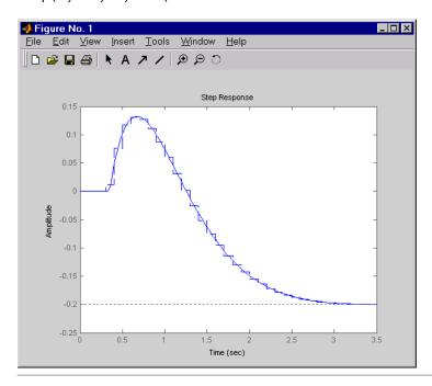
Discretize the delayed transfer function
