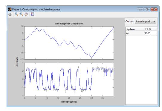
sys provides a 98.35% fit for the angular position and an 84.42% fit for the angular velocity.
