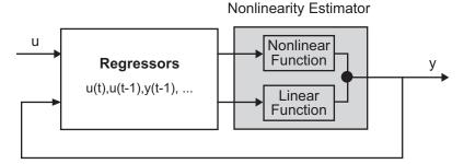
The nonlinear ARX model computes the output *y* in two stages:
