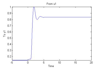
The model step response is a steady-state value of 0.8383 at T = 20 seconds.
