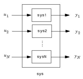
For systems with transfer functions  $H_1(s),\ldots,H_N(s)$ , the resulting system sys has the block-diagonal transfer function
