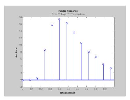
The first significantly nonzero response value occurs at 0.24 seconds, or, the third lag. This implies that the transport delay is 3 samples. To generate a model where the 3-sample delay is imposed, set the transport delay to 3:
