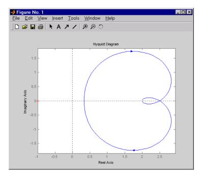
The nyquist function has support for M-circles, which are the contours of the constant closed-loop magnitude. M-circles are defined as the locus of complex numbers where
