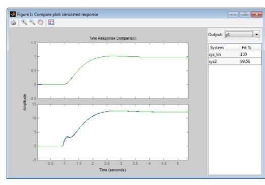
sys2 provides a 99.93% fit for the first output and a 98% fit for the second output while using 4 less states than sys lin.
