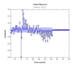
The large response value at t=0 (zero lag) suggests that the data comes from a process containing feedthrough. That is, the input affects the output instantaneously. It could also be that there is a direct feedback effect (proportional control without some delay that u(t) is determined partly by y(t)).
