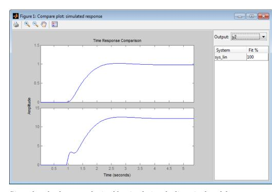
Given that the data was obtained by simulating the linearized model, there is a 100% match between the data and model linearization response.
