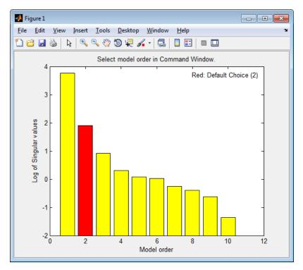
The plot shows the Hankel singular values (SVD) for models of the orders specified by nx. States with relatively small Hankel singular values can be safely discarded. The default order choice is 2.
