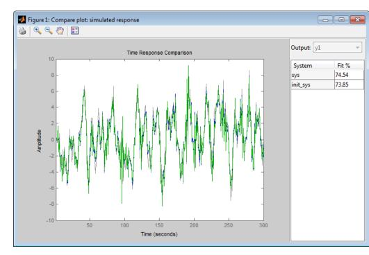
sys refines the estimated model and provides a 74.54% fit to the estimation data (see init sys.Report.Fit.FitPercent).
