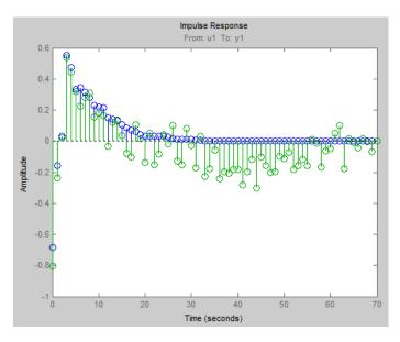
As the plot shows, using regularization makes the response smoother.
